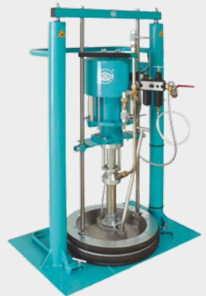
Pump unit with dual-post ram for 200 liter drums. We also offer ram units with a particularly large cylinder diameter for use with very high-viscosity materials.
